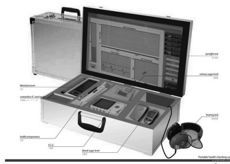
Fig. 6: $300 portable clinic. All the functions in a booth (in Fig. 4) can be designed and mounted in a suitcase. A grameen nurse can visit patients' home.
